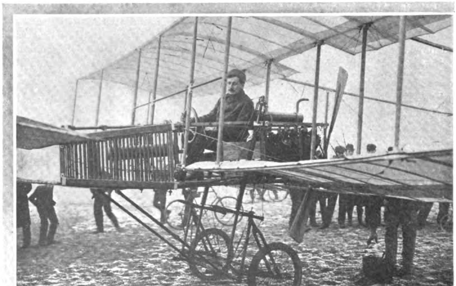
DELAGRANGE AEROPLANE, WITH EIGHT-CYLINDER ENGINE AND RADIATOR FORWARD.
